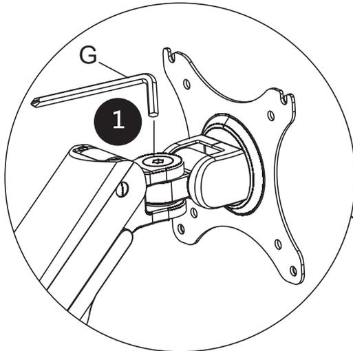
Use Allen Key (G) to adjust the swivel function on position 1
