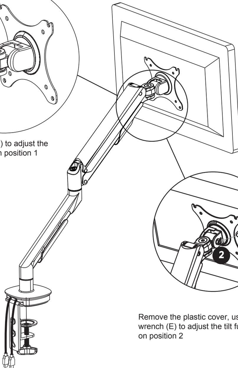
Remove the plastic cover, use box wrench (E) to adjust the tilt function on position 2
