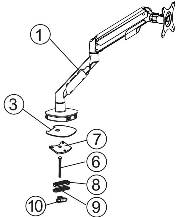
Choose proper grommet screw ⑥ based on thickness of desk:
